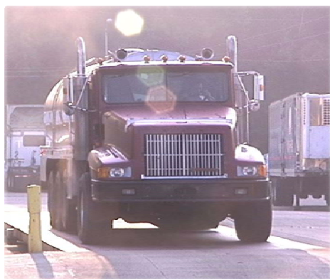
Truck scale operators should ensure a truck scale reading “stabilizes” prior to obtaining the scale weight reading.
