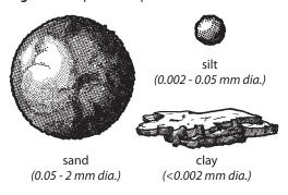
Although all of these particles seem small, the relative difference in their sizes is quite large. If a typical clay particle were the size of a penny, a sand particle would be as large as a house.
