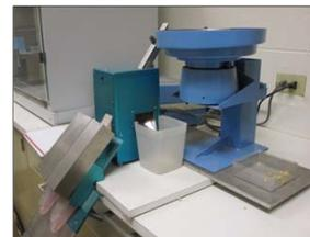
**Laboratory Seed Counter Operation** - The working sample is placed into the vibrating hopper of the seed counter. Seeds move through the carousel and are directed into a chute. As seeds pass through the chute, a light beam is broken. Each disruption is recorded and the number of seed per pound is calculated from the number of seeds recorded in the sample weight.
